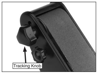
Figure 10. Sanding belt tracking knob.
